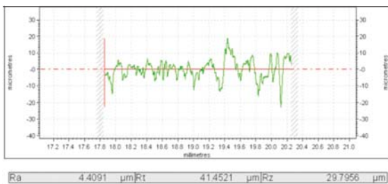
(b) f=100 mm/min, N=5000 rpm, d=4 mm
